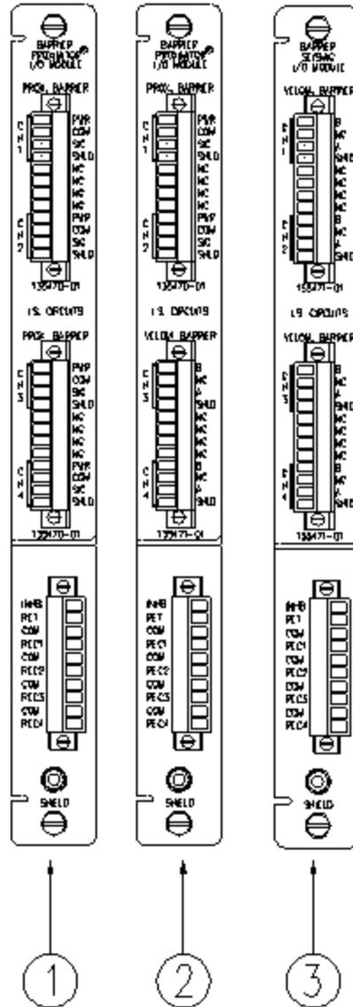
1. Barrier I/O Module for connecting four proximitor sensors
