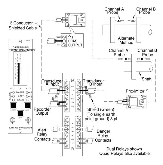
Field wiring diagram for 3300/47 Complementary Input Differential Expansion Monitor
