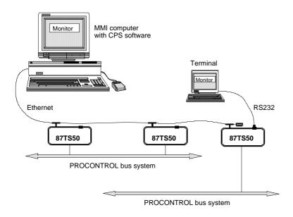
1 ... 4 87TS50 modules, optionally allocated to different PROCONTROL bus systems using different system addresses
